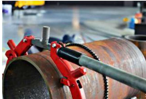
The Macstroc Rotary pipe cutter, designed for extremely low clearance and up to 36-inch pipe diameter, efficiently cold cuts steel, galvanized, and black iron pipes in tight spaces without producing debris, sparks, or significant heat, delivering a precise cut suitable for confined spaces such as trenches, underwater environments, noise-sensitive areas, overhead applications, and pipe racks.
